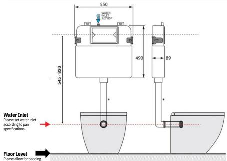
Please allow for bedding and tiles. Height to be set to finished floor level specifications.
